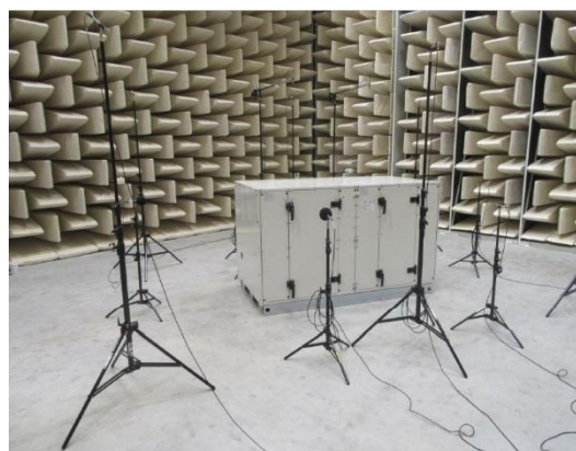
Fig. 2. Model box – acoustic chamber
