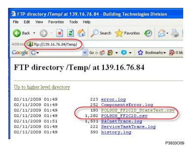
The EDE files are then used for offline integration, but could also be open in Excel to view what BACnet objects that are present.
