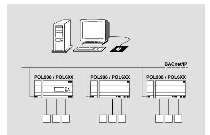
Climatix™ BACnet/IP communication with POL908.00 Integration guide
