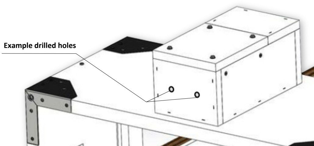
Example of position of holes in the wall of the box, without pre-manufactured slot
