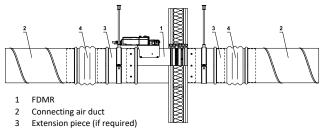
Extension piece (if required)Damping pad or breakaway connection as DW
