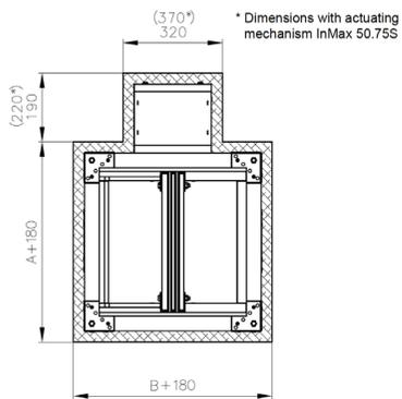
Insertion depth typically 250 mm for dampers supplied with flanges, and 200 mm for dampers without.
