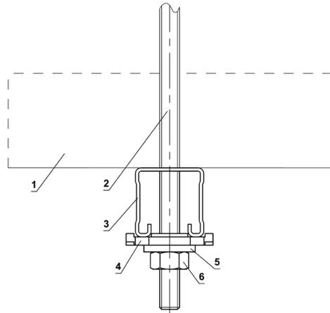
Drop rod and hanger position is not critical and can be positioned to suit the particular installation, applying symmetry where possible.
