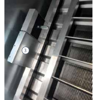
③ Actuating mechanism is always inside the chamber near the rear wall where there is a holder for its fixing
