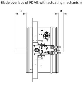
Blade overlaps of FDMS with VAV actuator
